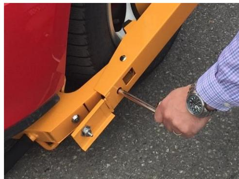
5. You may need to adjust the arm at the second crank point. Make sure the boot is held by the jaw and not the wheel cover and that the wheel cover is flush against the rim.
