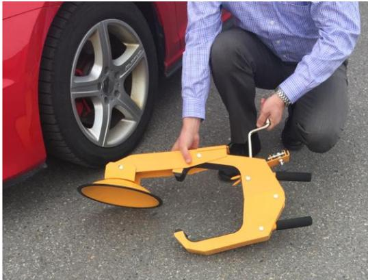
1. Use the key to unlock access to crank point
