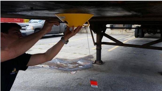
3. Screw the king pin lock on by turning screw clockwise. Make sure the handle is towards the back of the trailer
