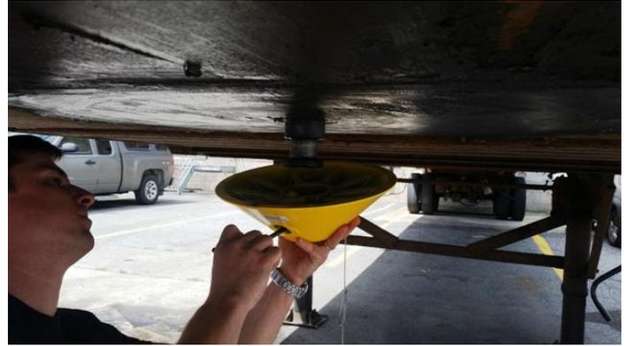
2. Using handle and allen key, lift king pin lock onto the trailer's king pin.
